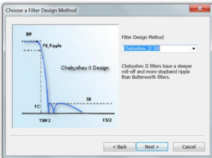
*Select the specific design method and enter the desired filter parameters in the next screen*
