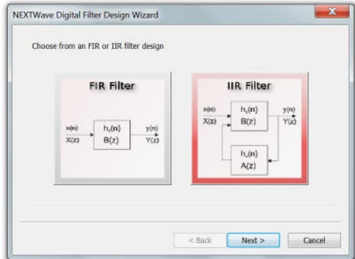
*The first step is to select the type of digital filter - FIR or IIR*
