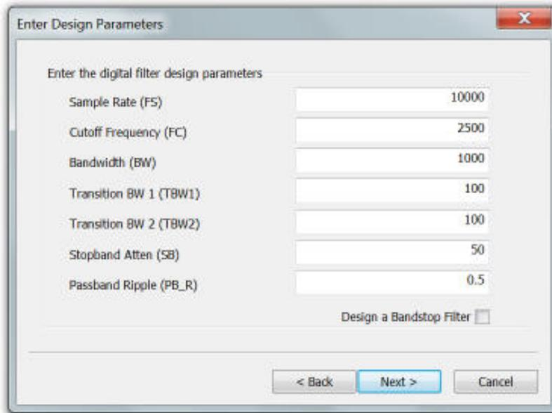
*Parameter Entry Screen for Digital Filter Design*
